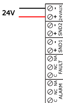
Fig. 15 24 V auxiliary output wiring
