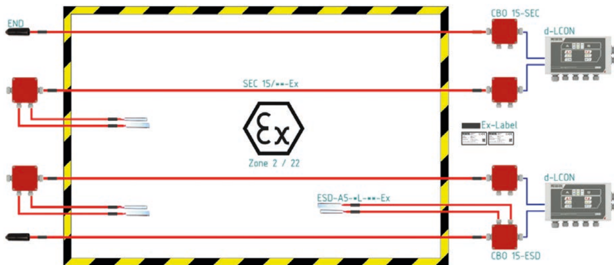
Fig. 3: Example 3: Installation of parts of the components in ATEX zones 2 / 22, sensor control unit d-LCON and connection boxes CBO 15-SEC, CBO 15-ESD as well as end caps END outside the ATEX zones
