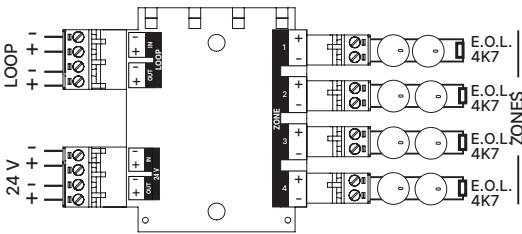
Up to 25 conventional detectors and conventional alarm buttons can be connected to the zone input.
